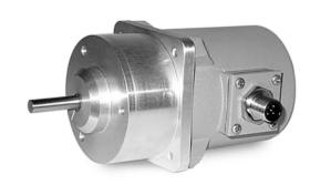
Celesco's model RT8DN communicates rotational position feedback via DeviceNET® to your programmable controller. The heart of this sensor is a precision plastic-hybrid position potentiometer which provides a "absolute" position and does not ever have to be reset to a "home" position after a power loss or planned shutdown.
