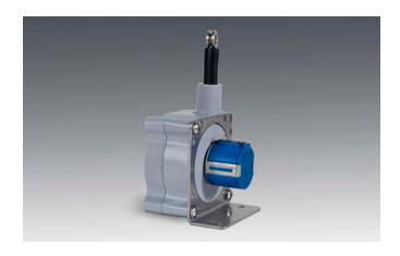
This compact stringpot with "voltage divider" output, provides the ultimate in ease-of-use and flexibility for measurement ranges up to 50 inches. Made of rugged polycarbonate, the SP1 fits in small spaces, doesn't need perfect alignment and ships with a stainless steel mounting bracket to let the user easily orient this sensor in just about any direction imaginable.
